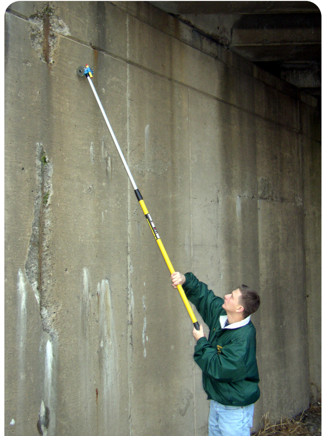
Delamination Detection Tool shown with attached crayon for on-the-spot marking of delaminated areas.
